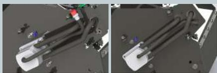
The machine comes standard in a two-pipe configuration, the fluidbox will manage the flow of oil coming from engine drainage. In the event that the back pressure at the discharge is greater than 8 bar, it's possible to provide for the third drainage tube for direct tank discharge.
