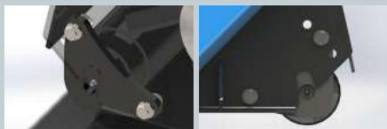
Rear support roller adjustable in three positions for cutting height adjustment.
