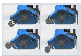
The rear idle roller can be configured in 6 distinct positions, which allow the volume and geometry of the case to be varied.
