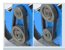
Transmission made with gear box and belts, possibility of inverting the pulleys for operation at 540 rpm or 1000 rpm.
