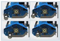
The rear idle roller can be configured in 6 distinct positions, which allow the volume and geometry of the case to be varied.
